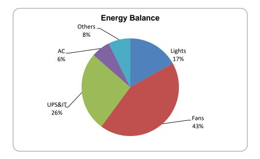
Fans account for 43% of the overall energy consumption in this facility, while lighting utilizes 17%, UPS and IT contribute 26%, and other miscellaneous uses constitute 8%. Additionally, 6% of the total energy is consumed by air conditioning systems.
